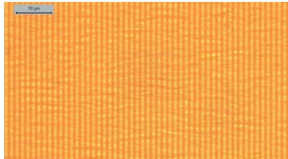
Microscope photo of a 50nm thin silicon film after scanning at 1.5\mu\text{m} pitch ( 515\text{nm} , 50\text{kHz} , 900\text{mJ}/\text{cm}^2 ).
